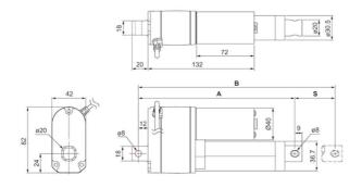
Bore tolerances: 8 mm  $^{+0,2}_{-0} \frac{mm}{mm}$
