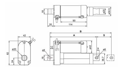
Bore tolerances: 8 mm  $^{+0,2}_{-0 mm}$
