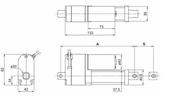
Bore tolerances: 8 mm +0.2 mm-0 mm
