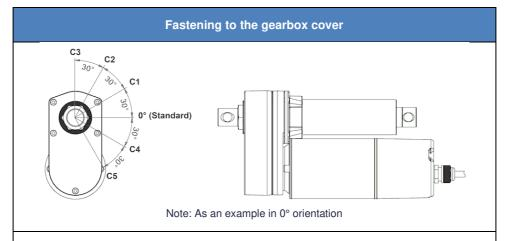
The mounting holes on the piston rod and on the gearbox cover are designed in the 0° orientation as standard. Optionally, a different angle (see picture) can be selected for the gearbox cover and piston rod. The angle between the selectable stages is 30° in each case.
